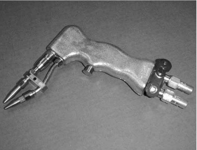
FIG. 15 The DHC 2000 Torch shown assembled for cutting sheet steel using the under cutter.
